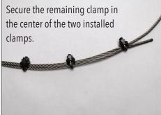
Orient the u-bolt on the "dead" end of the Retention Cable and the damp on the "live" portion of the retention cable. If done incorrectly, the U-bolt could crush the wire when tightened and can reduce the strength of the wire.
